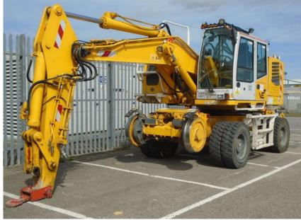
Built as a dedicated road-rail machine, the Colmar T10000 has class leading lifting capacity, beyond what would be achieved by converting a standard excavator for rail use.
