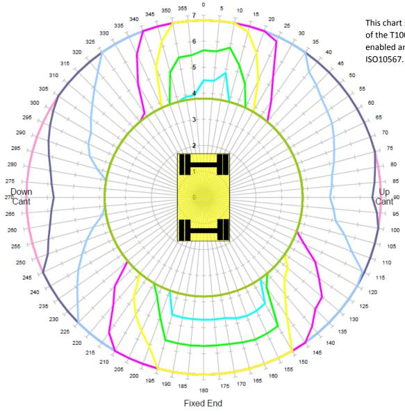
This chart shows the lifting capacity of the T10000 with the RCI system enabled and measures according to ISO10567.
