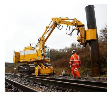
Built as a dedicated road-rail machine, the Colmar T10000 has class leading lifting capacity, beyond what would be achieved by converting a standard excavator for rail use.
