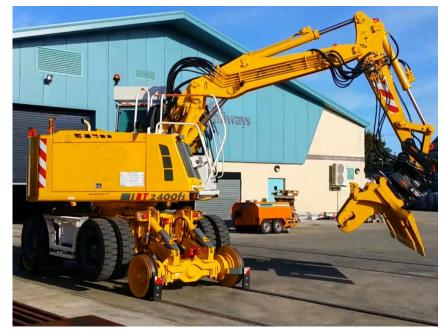
Built as a dedicated road-rail machine, the Colmar T2400 has class leading lifting capacity, beyond what would be achieved by converting a standard excavator for rail use.
